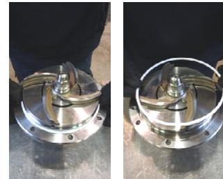
**Fig. 30** Retirer le joint (411.X) du support.
