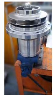
Fig. 34 Tighten the equipment (if available) in a bench vice and place the assembled bracket on top.
