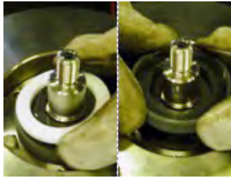
Fig. 38 Remove the compensation ring (504) and the front slewing bearing (510).
