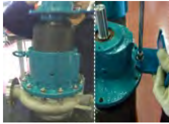
Fig. 30 Position the pump vertically. Loosen the screws (914) and separate the bearing bracket (330) from the pump using appropriate lifting systems. Loosen the screw and separate the foot (183) from the bracket (330).
