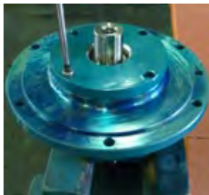
Fig. 53 Unscrew the oil bracket cover screws.
