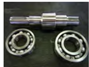
Fig. 58 Using the extractor to separate the bearings (321) from the primary shaft (213).
