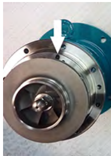
Fig. 66 Position the lubrication hole on the bushing bracket (350) as indicated.
