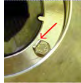
Fig. 64 For the "1st bracket" pumps: position the bushing locking flange (935) so that the anti-rotation tooth is aligned with the slot of the static bushing (545). Tighten the screws (901), bend and lock the washers. Turn the support (350) upside down and repeat the same operations to assemble the other static bushing (545).
