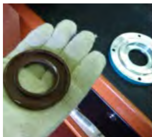
Fig. 56 Remove the oil seal (420) from the bearing cover (360).
