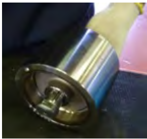
Fig. 41 Extract the secondary shaft (211) from the internal magnetic core (855).
