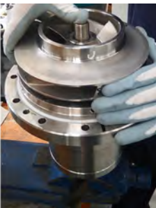
Fig. 35 Unscrew and remove: the impeller nut (922), the washer (931) and the impeller (230).
