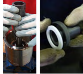
Fig. 40 Extract the following from the impeller shaft (211): the rotating bushing (529), the rear slewing bearing (510) and then the compensation ring (504).
