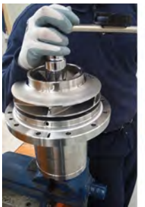
Fig. 35 Unscrew and remove: the impeller nut (922), the washer (931) and the impeller (230).
