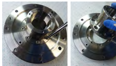
Fig. 48 For the "1st bracket" pumps: if the bushing bracket is divided (351 + 352), loosen the screws (914) and the washers (931) to separate the "flange" (351) from the seat (352).
