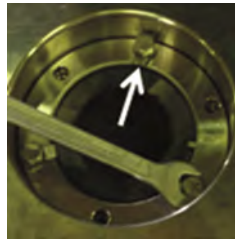
Fig. 45 For the "1st bracket" pumps: from the bushing bracket (350) disengage the safety washers indicated by the arrow (931) from the screws (901) and loosen the bushing locking flange (935).
