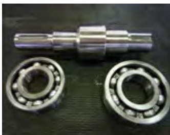
Fig. 68 Heat the bearings (321) using a specific heater and insert them on the primary shaft (213).
