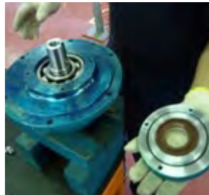
Fig. 54 Separate the cover (360) from the bearing bracket (330).
