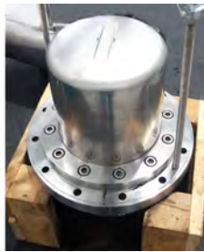
Fig. 32 Remove the assembled bracket from the volute casing (102) and place it on a stable spacer (do not "load" the impeller with the weight of the assembled bracket).
