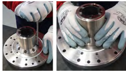
Fig. 42 For the "2nd bracket" pumps: loosen the screws (914) and the washers (931) to separate the "flange" (351) from the bushing bracket seat (352).
