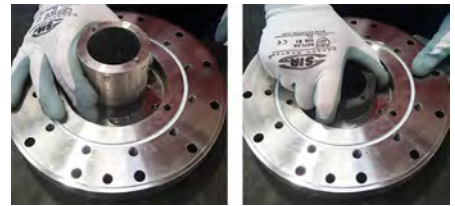
Fig. 43 For the "2nd bracket" pumps: extract the spacer ring (504) and the front static bushing (545).
