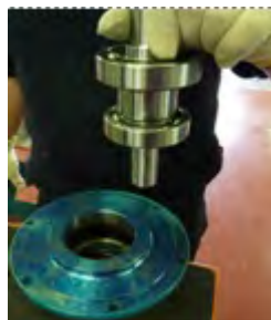
Fig. 57 Remove the primary shaft (213) and its bearings under the press.
