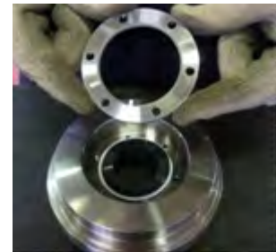
Fig. 46 For the "1st bracket" pumps: extract the bushing locking flange (935) from the bushing bracket (350).
