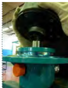
Fig. 51 Extract the outer magnetic core (856) from the primary shaft (213).
