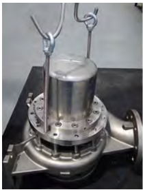
Fig. 32 Remove the assembled bracket from the volute casing (102) and place it on a stable spacer (do not "load" the impeller with the weight of the assembled bracket).
