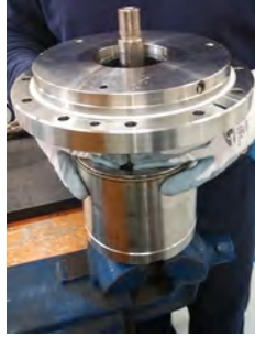
Fig. 39 Extract the bushing bracket (350).
