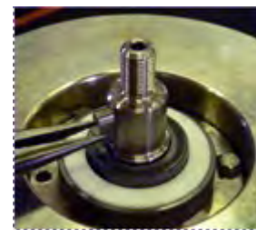
Fig. 37 Remove the front feather key (940) from the secondary shaft (211).
