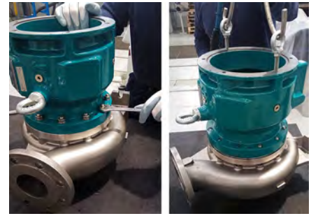
Fig. 31 Loosen the nuts (920) and separate the lantern (344) from the volute casing (102) using appropriate lifting systems.
