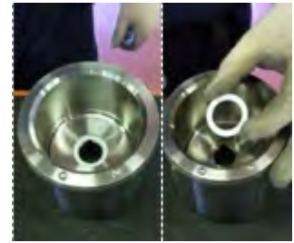
Fig. 49 Extract the gasket of the rotating bushing (411) from the internal magnetic core (855).
