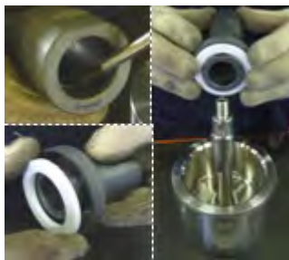
Fig. 65 Caution! Insert the components on the rotating bushing (529) from the side that has been internally milled as indicated. Insert: the rear thrust bearing (510), the axial clearance compensation ring (504). In the "high temperature" version, insert the reinforced Grafoil ring (504) into the thrust bearing (510) and then the metal shim (504). Insert everything on the secondary shaft (211).
