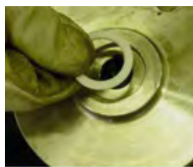
Fig. 36 Turn the impeller (230) upside down and extract the rotating bushing gasket (411).
