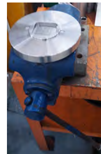
Fig. 34 Tighten the equipment (if available) in a bench vice and place the assembled bracket on top.
