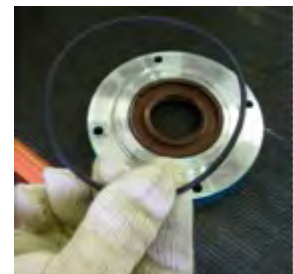
Fig. 55 Pull out the O-Ring (412) from the bearing cover seat (360).
