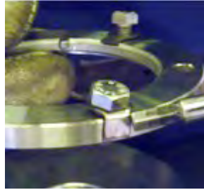
Fig. 63 For the "1st bracket" pumps: insert the hex head screws (901) and their safety washers (931) into the holes of the bushing locking flange (935) and bend the washers over the outer edge of the flange (935).
