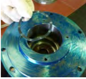
Fig. 59 Remove the compensation ring (500) from the bearing bracket (330). Turn the bearing bracket (330) upside down and repeat the operations in fig. 52 to separate the cover (360).
