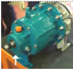
Fig. 29 Empty the oil contained in the bearing bracket by unscrewing the drain plug (912).
